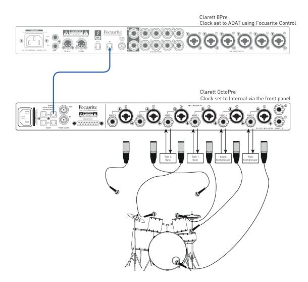
When recording acoustic drums, dynamics control may be applied in various ways to get the sound you're after. Compression is frequently added to kick and snare drums to thicken up the sound, while noise gates are effective on tom-toms to minimise spillage between the various drum mics.
