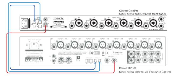
This example shows the same setup as Example 2, but running at a sample rate of 96 kHz ("SMUX-II" mode). Both units must be set to 96kHz; two optical cables are used, carrying four channels of audio each. The Clarett 8PreX is the sync master as before.
